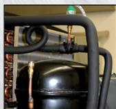
The thermal expansion capillary tube boosts performance and reactions in the system under all operating conditions.
