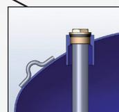
Magnesium sacrificial anode per DIN 4753 for perfect corrosion protection.
